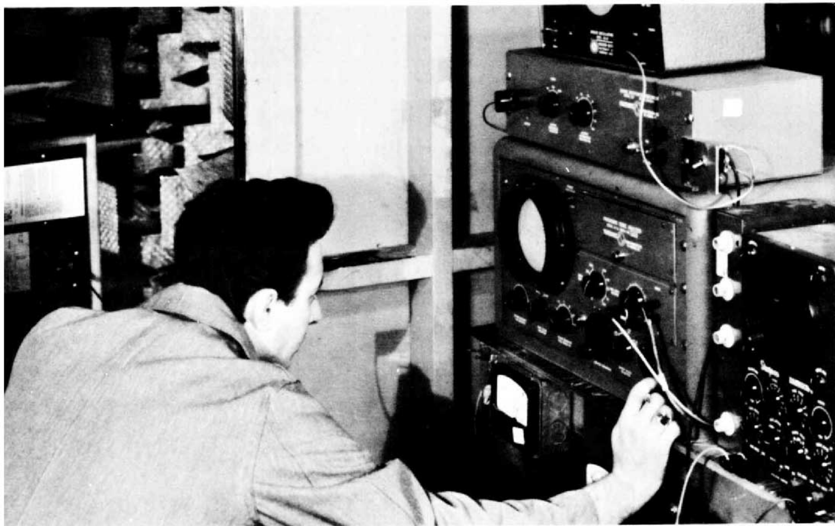
Silvano Cannavacciuolo, AR inspector, checks a speaker response curve at one of AR's anechoic chambers. The response curves of the individual drivers in the system he is testing have already been recorded and found acceptable at the main anechoic chamber.
